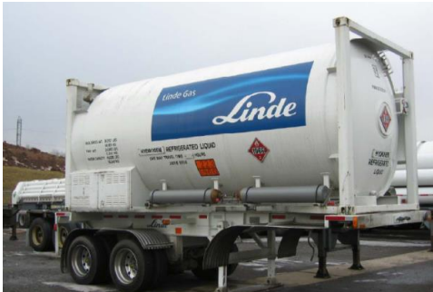
LH 2 Storage Tank on Trailer
